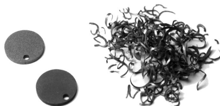
Fig. 1 Samples - titanium discs and turnings used for exposure in SBF
